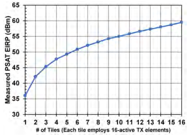
Fig. 25. Measured saturated EIRP at 90.7 GHz as a function of active tiles.
