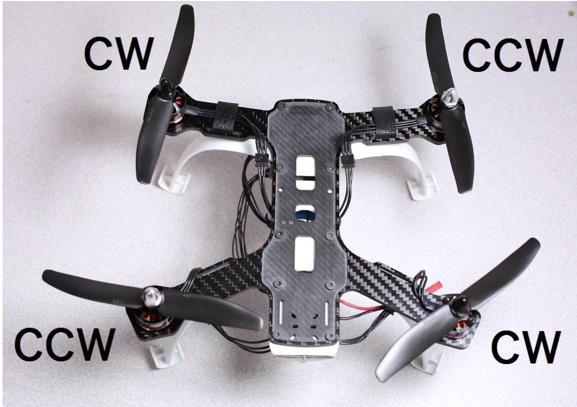
Figure 2.18—Mounting the propellers
