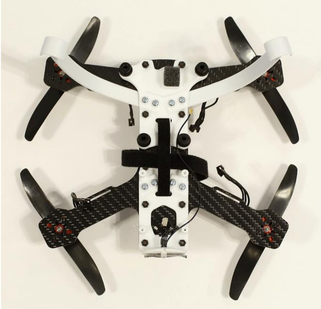
Figure 2.1—Mounting the front landing gear
