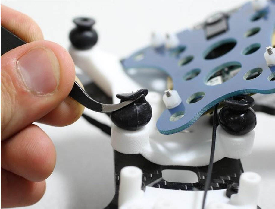
Figure 2.9—Squeezing the neck of the damper
