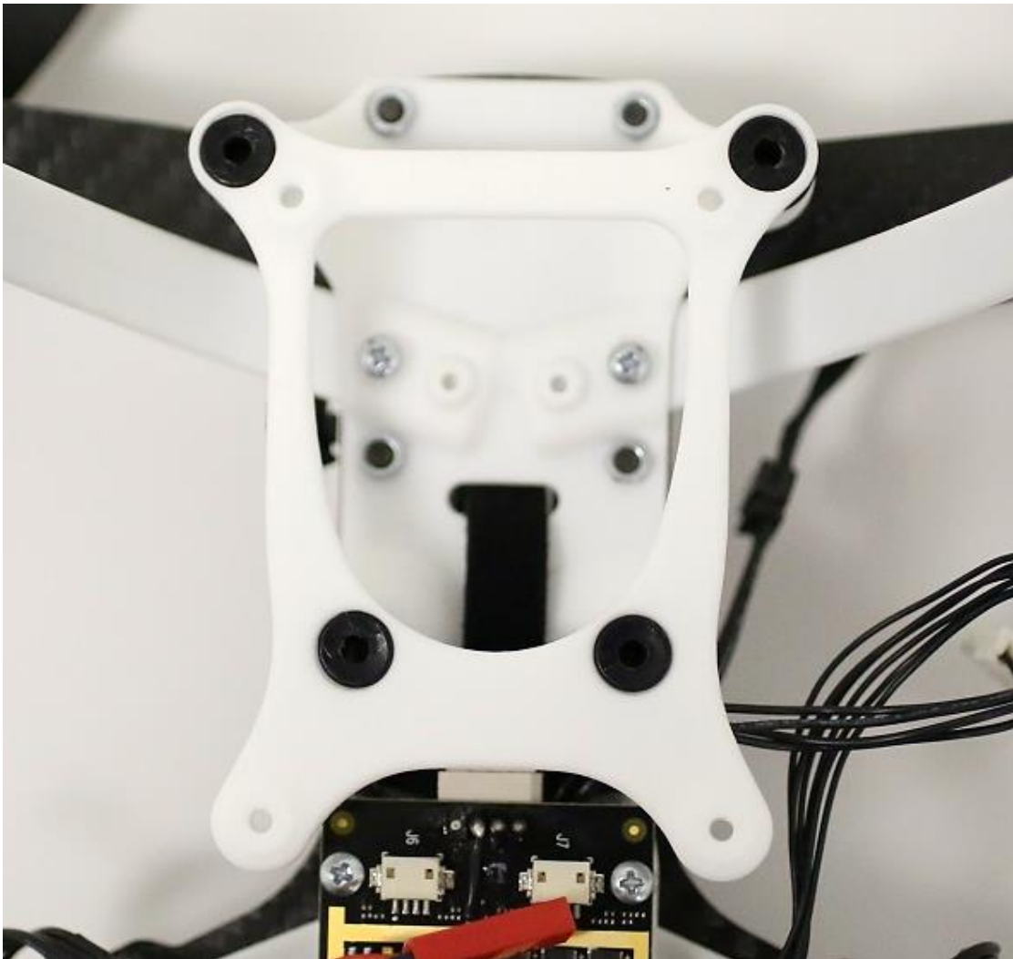
Figure 4.1—Inserting the dampers into the stereo adapter
