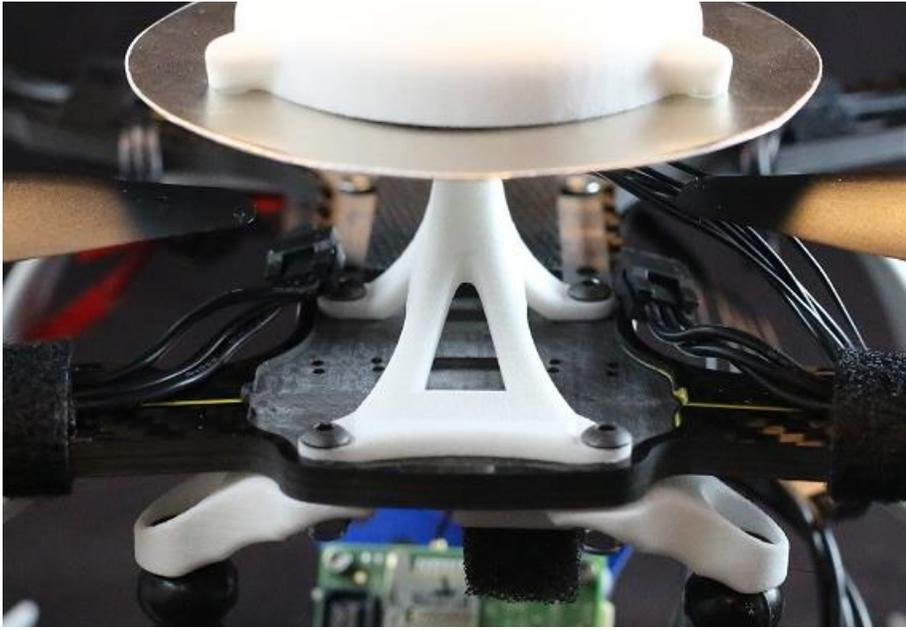
4. Reinsert the two landing gear, first loosening the set screws in the Snapdragon Flight™ Adapter, and then retightening them so that the landing gear are secure.
