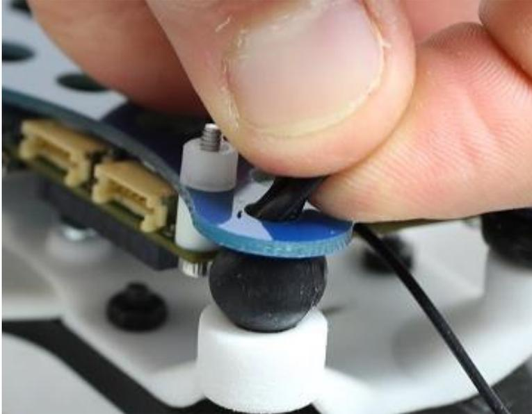
8. Repeat this process for the other three dampers until they are each fully inserted into the blue mount plate, as visible below. Note the gray foam protruding from the Snapdragon Flight™ Adapter, and make sure that it fits straight down onto the circuit board. This covers the barometer to ensure that it is protected from light interference.
