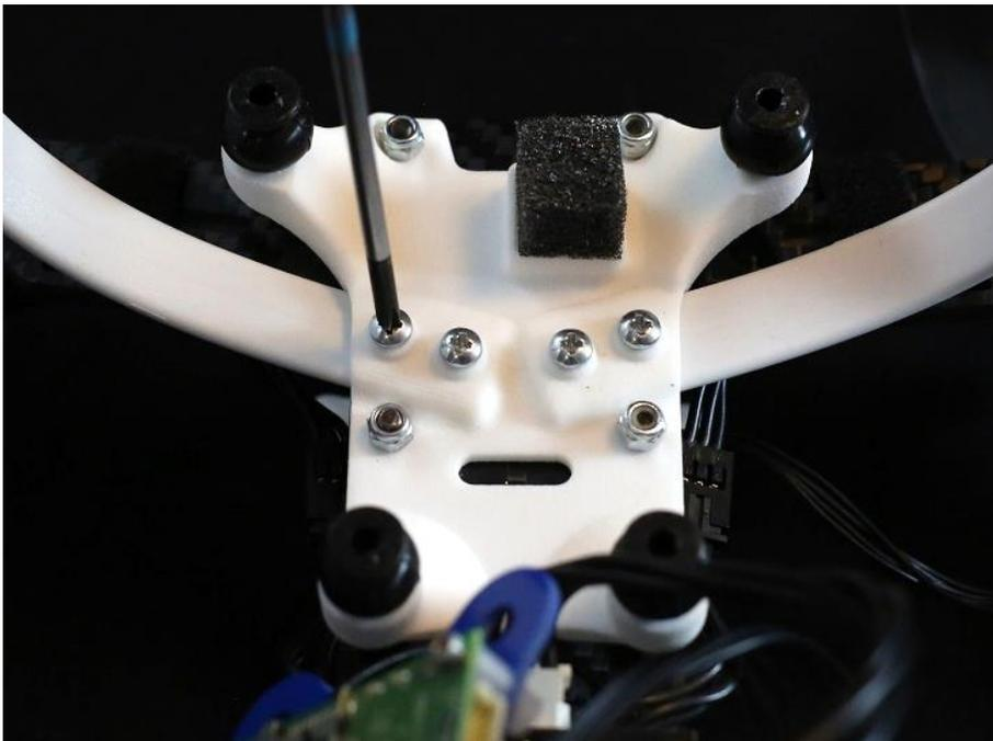
5. The next step is to reattach blue plate on which the Snapdragon Flight™ board is mounted to the dampers. To do this, pinch the neck of one of the dampers curved tweezers such that the end of the tweezers lines up with the end of the damper, as shown below.
