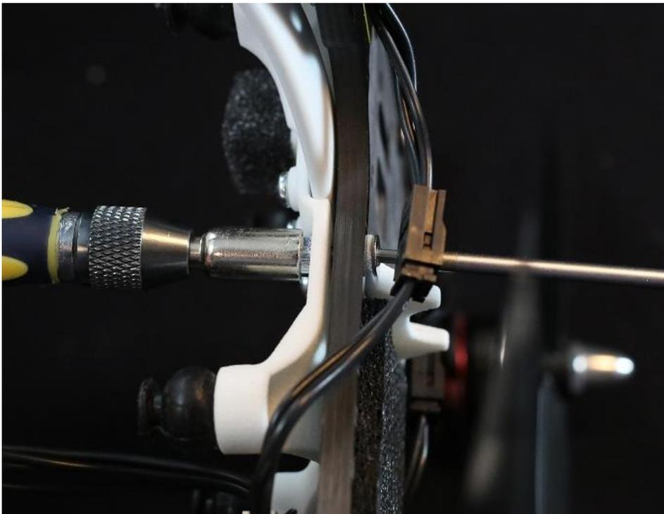
3. Align the GPS Mount with the four holes on the top of the frame from which the screws were just removed such that the vertical face of the mount faces back toward where the battery rests, as shown below. Realign the loose Snapdragon Flight™ Adapter in its original position, and insert four M3x12mm screws into each of the four holes of the GPS mount, securing them with the original nuts.
