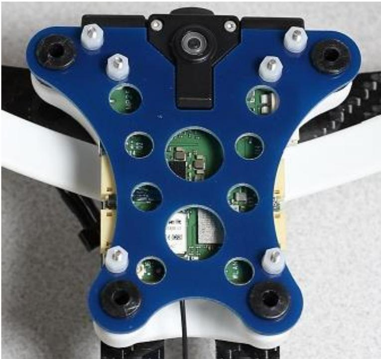
9. Finally, route the GPS cable through the hole in the center of the mount and out the left side, as pictured in the following photo. This ensures that the cable will not come into contact with the propellers while they are spinning. Plug the cable into the connector next to the power connector on the Snapdragon Flight™, as indicated with the yellow arrow below.
