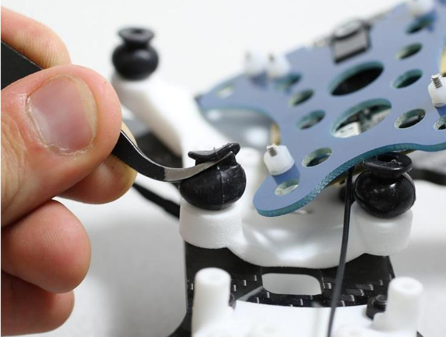
6. Insert the squeezed end of the damper through the large hole in the corner of the blue mount plate such that the Snapdragon Flight™ board is down, toward the adapter and frame, as illustrated below. Be careful not to puncture or rip the damper during this process.
