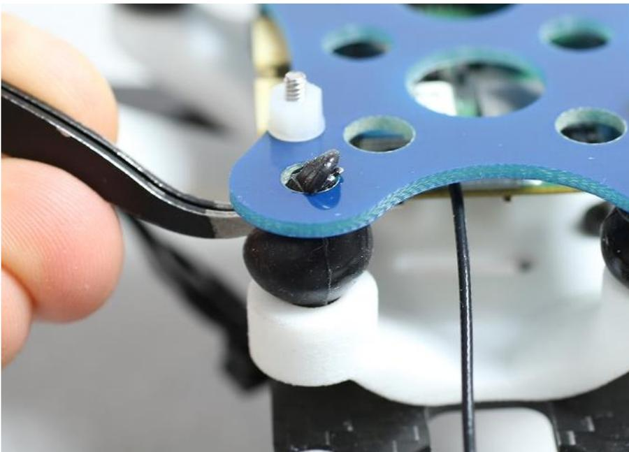
7. Once the damper is poking through, grab the other end with fingers and begin to pull it through the hole, as shown in the example below. Continue to pull and reposition the top flange until it is entirely through the hole and rests flat on the other side of the blue mount plate.
