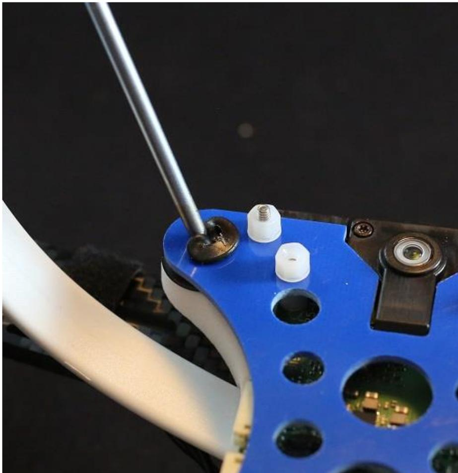
2. Remove all four screws holding the Snapdragon Flight™ Adapter in position, as indicated in the two pictures below. Note that the front two landing gear will be loose once the adapter is removed. Remove them along with the adapter.
